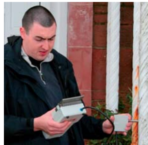
Dr Craig Kennedy, one of the NHSS steering group members undertaking hand-held Raman spectroscopy to analyse the paint on the surface of a cast iron canopy in Rothesay, Bute, Scotland.
